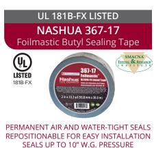
SEAM, SEAL, AND JOIN CLASS 1 FLEXIBLE DUCT. SEALS RIGID SHEET METAL DUCT JOINTS INCLUDING SLIPS & DRIVES.
